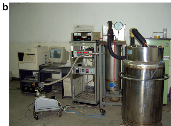
Fig. 1. Experimental apparatus, (a) schematic diagram (b) photo: (1) boiling vessel, (2) refrigerants tank, (3) liquid-nitrogen cryostat, (4) vacuum chamber, (5) copper cylinder, (6) condenser, (7) electric heater, (8) pressure transducer, (9) electric-magnetic valve, (10) platinum resistance thermometers, (11) gas chromatograph instrument.
